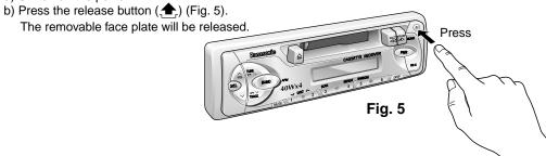
c) Remove the removable face plate by pulling on the right side of the unit. Place the removable face plate in a supplied case.
